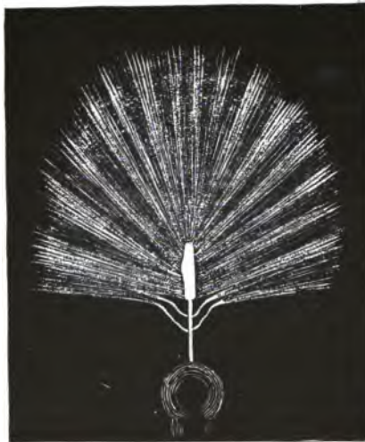
Diffused brush discharge of electrical machine, when operating with its current cut off or interrupted between machine and principal condenser.
